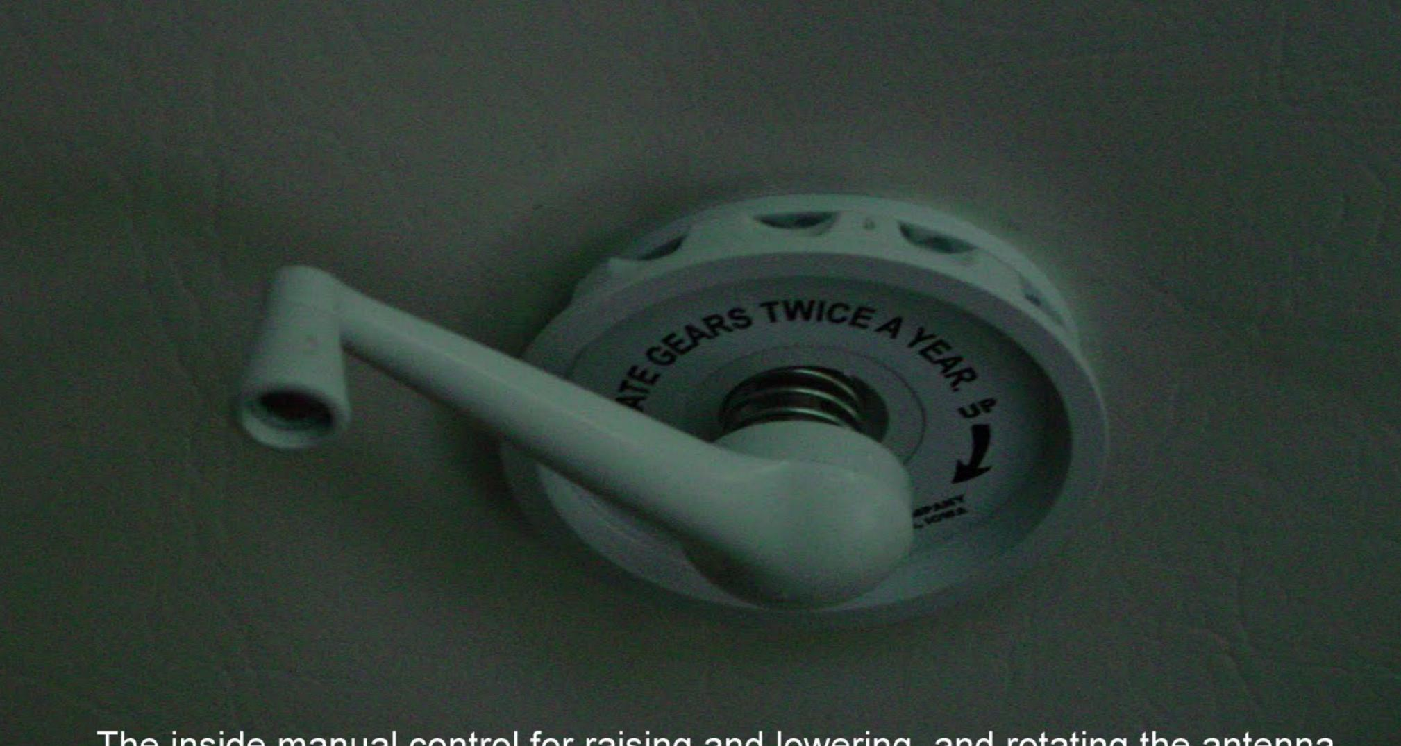
The inside manual control for raising and lowering, and rotating the antenna. Extra care must be taken to properly position the detent plate mounted to the inside roof.
