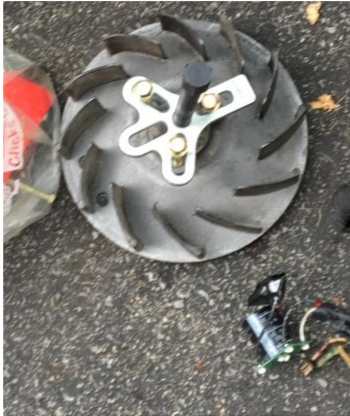
*Illustration 5: Fan Hub Assembly with Harmonic Balance Puller attached*
