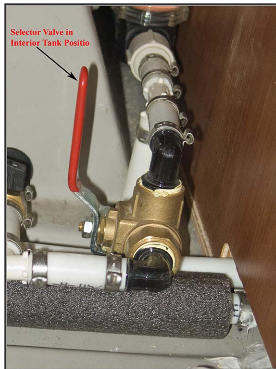
Picture W-13: Selector valve position for supply from the interior fresh water tank.
