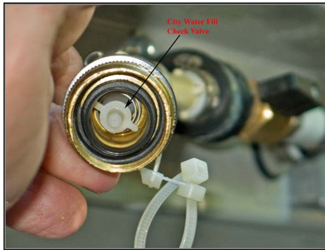
Picture W-19: City water fill check valve.
