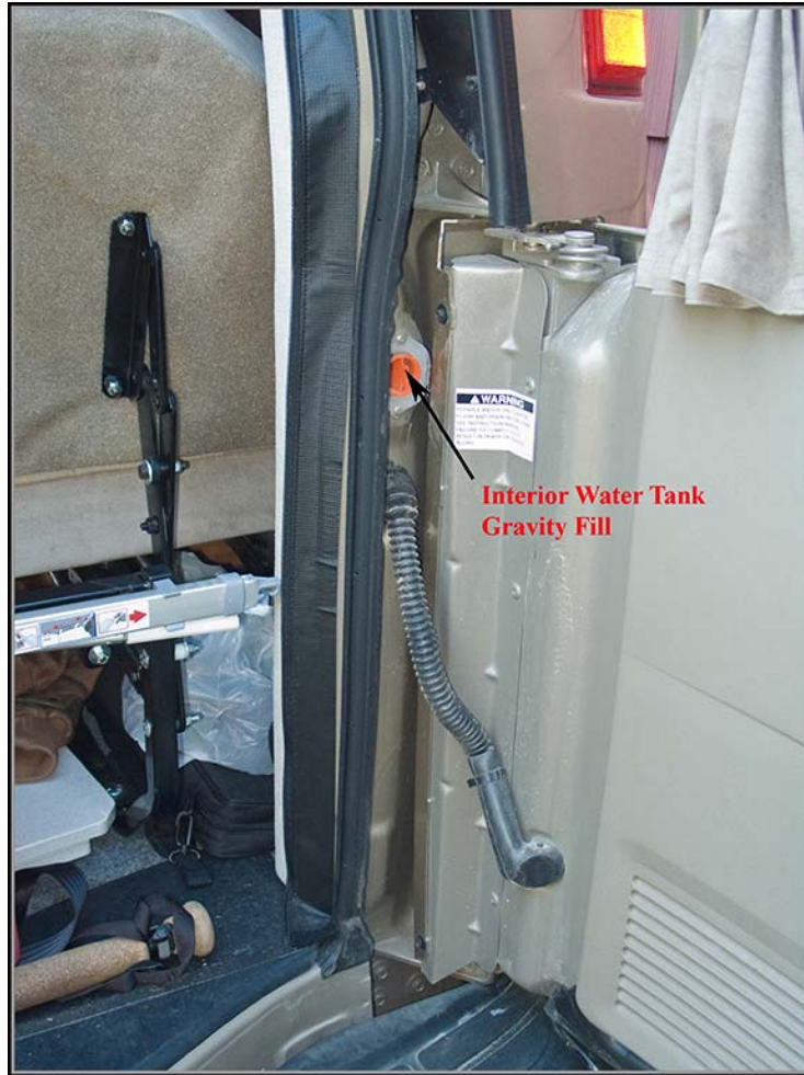
Picture W-3 : The gravity fill for the interior fresh water tank, (located on passenger-side rear door post).
