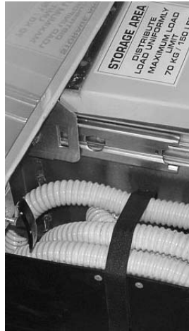
Picture G-P17: Sewage discharge hose storage located in driver's side storage drawer.
