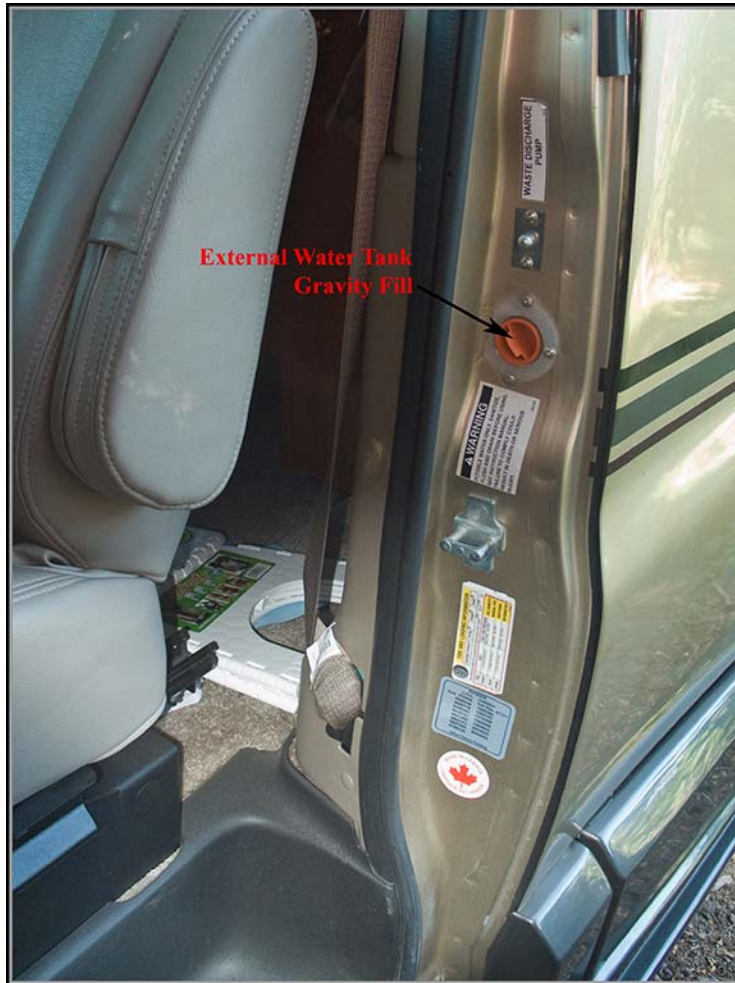
Picture W-4: The water fill for the external fresh water tank, (located at driver-side front door post).
